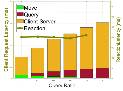
Figure 3.17: Latency breakdown with increasing query ratio under Freshness semantics.
