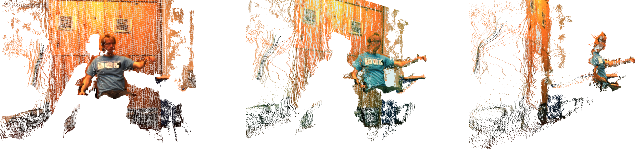
Fig. 6 A rendering of the data from the stereo camera from different views.
