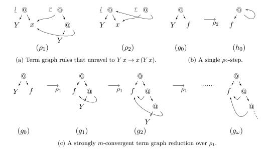
Figure 1: Implementation of the fixed point combinator as a term graph rewrite rule.
