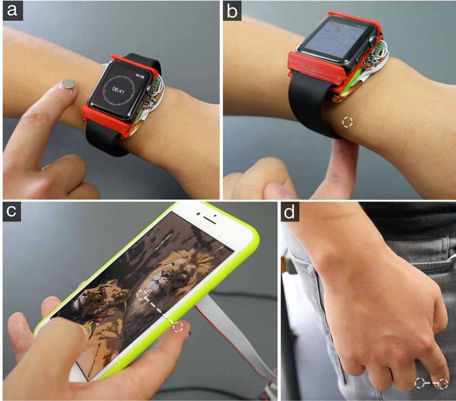
Figure 11: Magnetips enables these interactions: a) 3D mid-air, b) Behind arm, c) Back of device, d) Through material.
