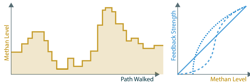
Figure 66: Interaction in the Cognitive Band as the user walks through Tidmarsh, the levels of methan vary (left). Based on the methan concentration the amplitude of the vibrotactile feedback is adjusted (right).
