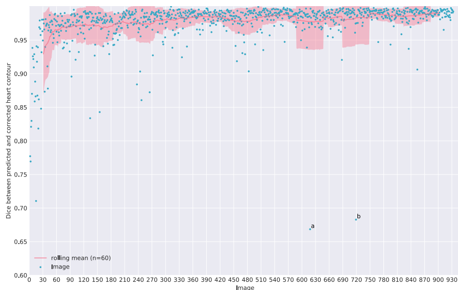
Figure 3.6: The dice score for 933 images shown in delineation order. The dice score compares the predicted vs. the corrected contour for each delineated heart. After the initial training period, the vast majority of dice scores are above 0.9, with only a few outliers dropping below. Outliers are labelled a and b.
