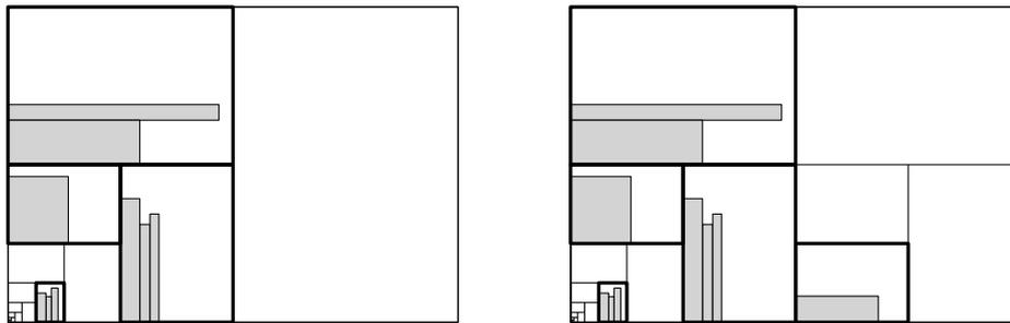
Figure 4.1: Left: Rectangular pieces packed into bricks. Right: A new piece arrives and it is packed in a brand new brick. The brand new brick is picked so that is the smallest that can host the new piece.
