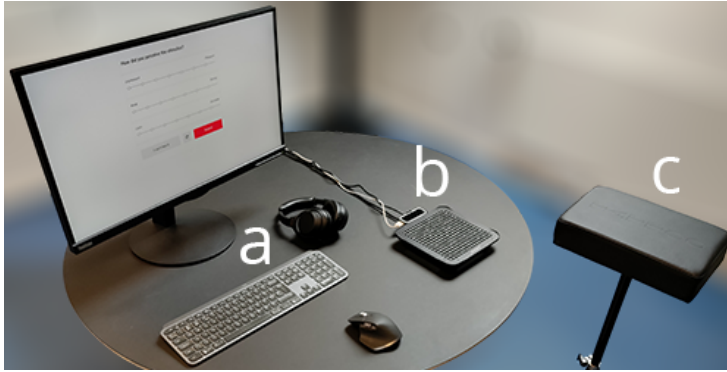
Figure 6.3. The setup in the first study, consisting of (a) a screen, keyboard, mouse and headphones; (b) the mid-air haptics device STRATOS Explore and Leap Motion controller; (c) and an armrest.
