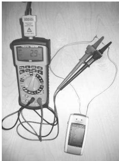
Figure 2: Setup for the measurement: We measure the voltage drop over a resistor inserted in series between the battery and the mobile phone
