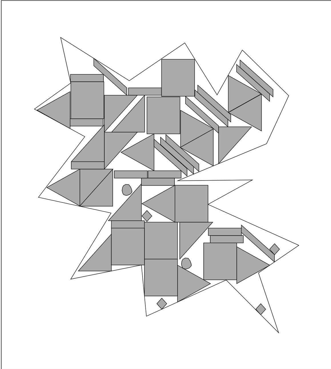
Figure 7.4: An example of nesting inside an irregular material. It should be noted that this is not a difficult nesting problem — it was found within 10 seconds using the implemented nesting solver.
