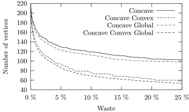
Figure 8.3: The number of vertices left in the Swim instance when different levels of waste are allowed.
