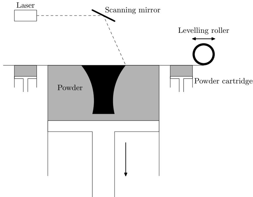
Figure 2.5: An example of a typical machine for rapid prototyping. The powder is added one layer at the time and the laser is used to sinter what should be solidified to produce the objects wanted.
