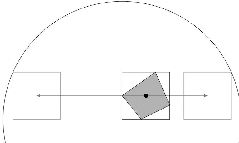
Figure 7.5: Keeping polyhedra within the boundaries of a cylinder can as a rough approximation be reduced to the problem of keeping a bounding box inside a circle.
