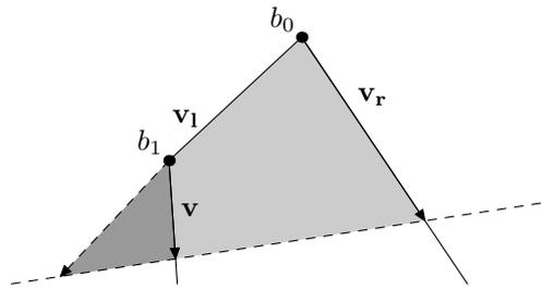
Figure 6.7: At each breakpoint after the initial breakpoint(s) the shape changes. This can be handled subtracting a new growing area (dark area) from the existing growing area (light and dark area).
