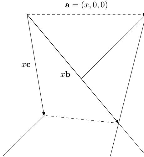
Figure 6.3: The volume of the above tetrahedron can be calculated from the three vectors  $\mathbf{a}$ ,  $\mathbf{b}$  and  $\mathbf{c}$ . In our case  $\mathbf{b}$  and  $\mathbf{c}$  are linearly dependent on  $x$  which is the length of  $\mathbf{a}$  (and the translation distance since the tetrahedron started growing).
