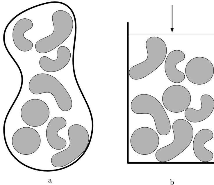
Figure 2.1: a) Most variants of the nesting problem is the problem of packing shapes within some region(s) without overlap (decision, knapsack and bin packing). b) The strip packing variant asks for a minimization of the length of a rectangular region.
