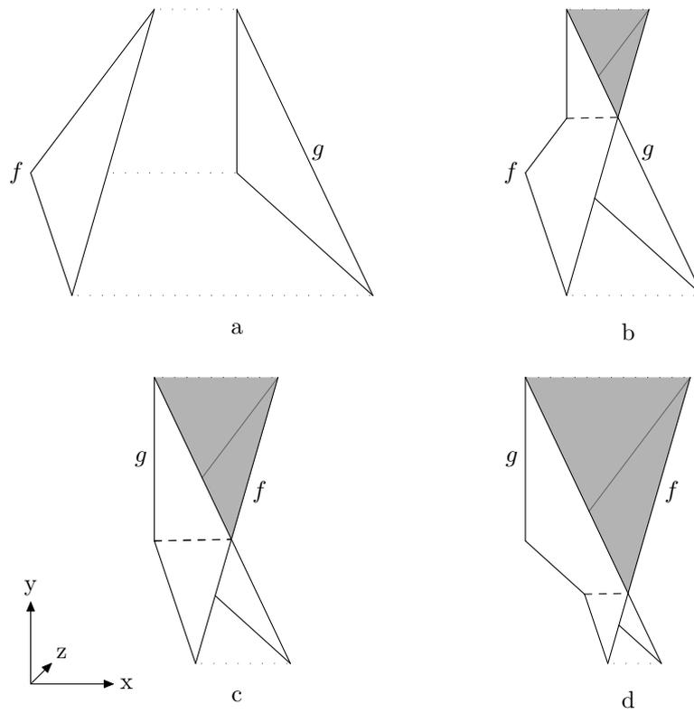
Figure 6.2: The  $x$ -translation of a triangle  $f$  through another triangle  $g$ , where the triangles have the same projection onto the  $yz$ -plane. The region volume  $R(f, g)$  changes shape each time two corner points meet.
