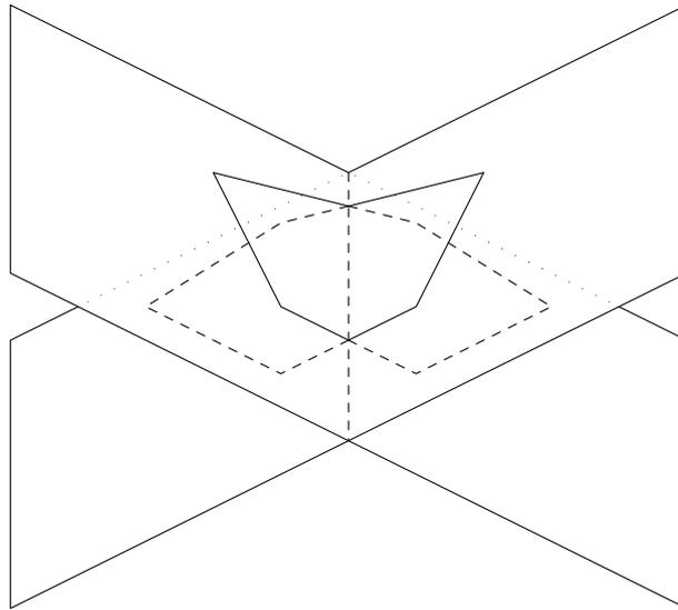
Figure 6.4: Just like two non-parallel planes have a single unique line in common so will two crossing faces have a unique line segment in common.
