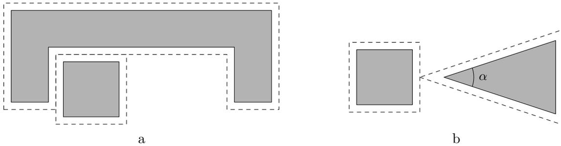
Figure 5.4: a) A simple enlargement of two polygons can guarantee some required minimal distance between them. b) A simple enlargement can force polygons to be farther apart than necessary
