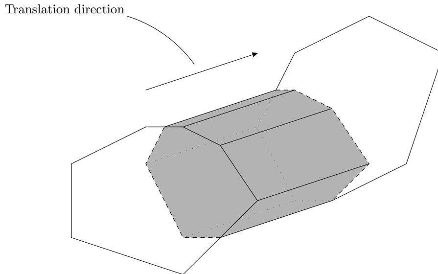
Figure 6.1: An illustration of the region volume between two faces. The faces are not necessarily parallel, but the sides of the region volume are parallel with the translation direction. The region volume would be more complicated if the two faces were crossing.
