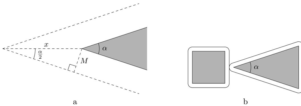
Figure 5.5: a) The distance  $x$  should be close to the distance  $M$ , but this is clearly not the case. b) The problem can be solved by rounding the corners
