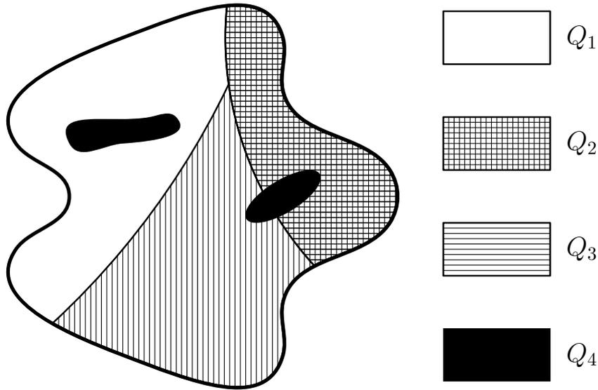
Figure 5.3: A piece of material, e.g. an animal hide, can have areas with different levels of quality. The stencils to be placed can have different quality requirements — even a single stencil can be divided into areas with specific quality requirements.
