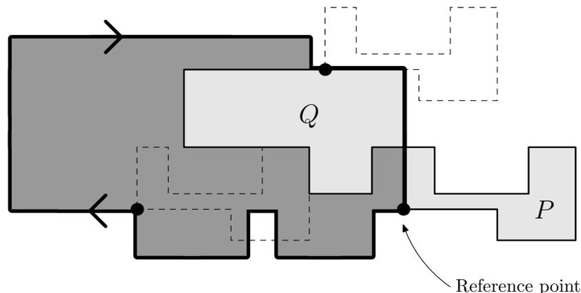
Figure 2.3: Example of the *No-Fit-Polygon* (thick border) of stencil  $P$  in relation to stencil  $Q$ . The reference point of  $P$  is not allowed inside the NFP if overlap is to be avoided.
