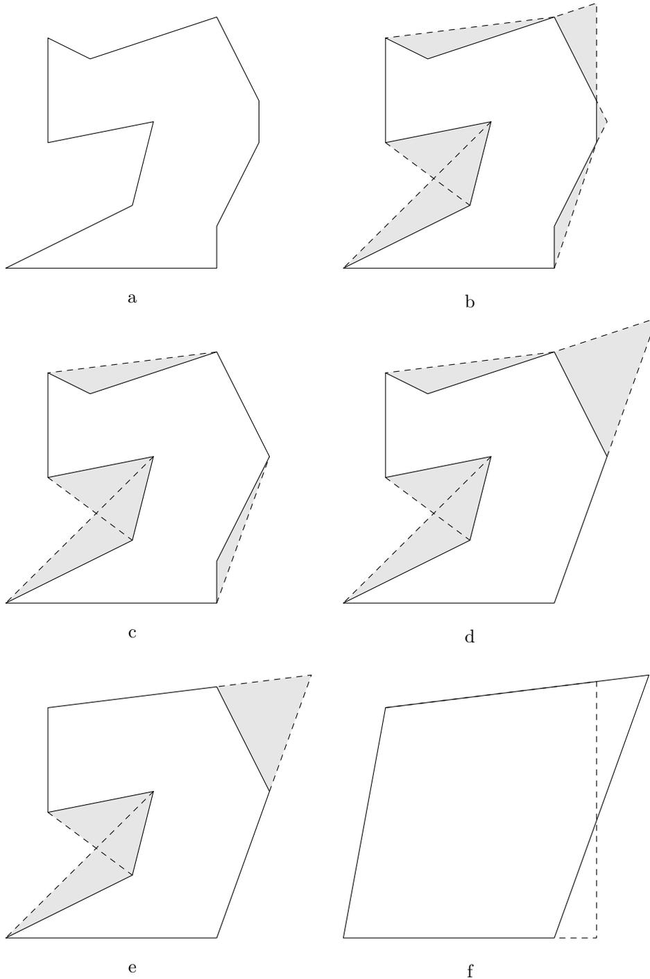
Figure 7.7: a) A highly irregular polygon with 11 vertices. b) The set of all border triangles which it is possible to remove. 2 convex and 5 concave border triangles. c-e) The triangle of smallest area is iteratively removed. The list of border triangles is updated at each step. f) Continuing as long as possible results in a polygon with just 4 vertices and naturally no concavities. The dashed line indicates a quadrilateral with smaller area not found by the algorithm.
