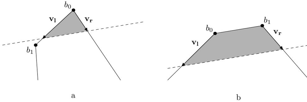
Figure 6.6: Two situations need to be handled at the initial breakpoint. a) The intersection line meets a single breakpoint  $b_0$  and “grows” a triangle. b) The intersection line meets two breakpoints simultaneously and “grows” a quadrilateral.
