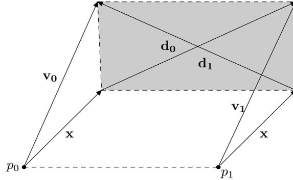
Figure 6.8: It is necessary to also be able to calculate the volume of a growing pentahedron as the one above. Note that  $\mathbf{x}$  is a vector parallel to the  $x$ -axis. Its length is the translation distance.
