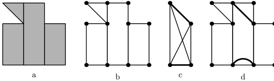
Figure 5.8: Various steps in the process of finding a shortest cutting path. a) A given nesting solution. b) A graph corresponding to the edges which need to be cut. c) The odd nodes of the graph with all vertices connected. The thick lines show a minimal 1-matching. d) The edges from the 1-matching is added to the original graph revealing a graph with even nodes only. A solution is now easily found.
