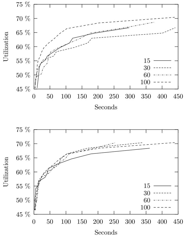
Figure 8.5: Experiments with bounded translation of stencils. The curves represent 15%, 30%, 60% and 100% translation relative to the maximum translation distance. Swim was used in both of the above experiments, but the latter also used approximated stencils.
