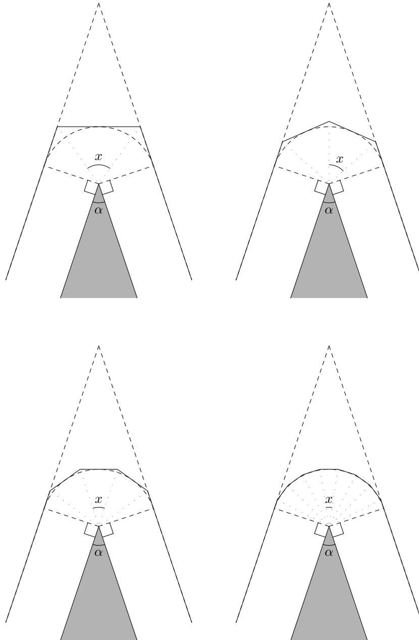
Figure 5.6: Examples of approximated rounded corners using 2, 3, 4 and 8 extra vertices. The dashed circular arc is the optimal enclosure.
