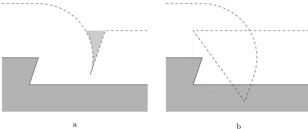
Figure 5.7: a) A naive rounding of corners can cause the resulting polygon to be illegal in the sense that the margin is no longer guaranteed. b) A subtle fix to this problem is the addition of two points for each concave corner (and a removal of the self intersection).
