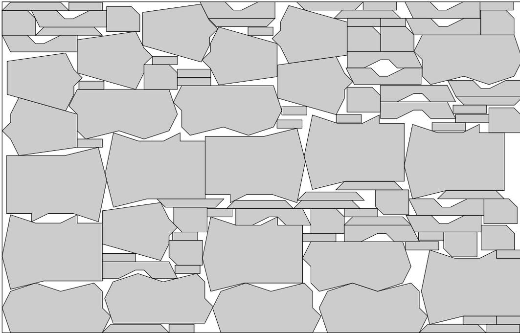
Figure 1.1: A tight packing using 86.5% of the available area (generated by 2DNEST developed for this thesis).
