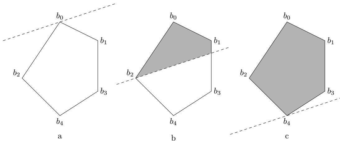
Figure 6.5: This is a 2D illustration of the process of two faces (with identical 2D projections) passing each other. The dashed line is the line of intersection from Figure 6.4. a) The first breakpoint when the two faces meet for the first time. b) At  $b_2$  the projected polygon is given by all previous breakpoints and the intersection line. c) At  $b_4$  the two faces have passed through each other entirely.
