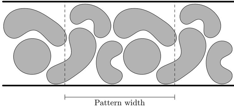
Figure 5.2: An example of repeated pattern nesting in 1 dimension. The pattern width is to be minimized, but unlike strip packing the stencils can wrap around the vertical limits.
