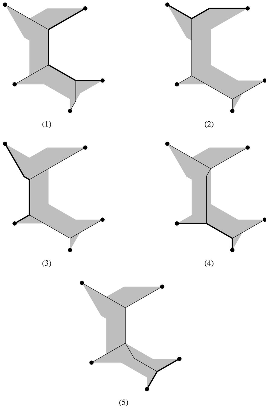
Figure 10: Rightmost concave paths defining a flexibility polygon for  $\lambda = 6$ . For each rightmost concave path, a  $\lambda$ -SMT realizing this path is shown.
