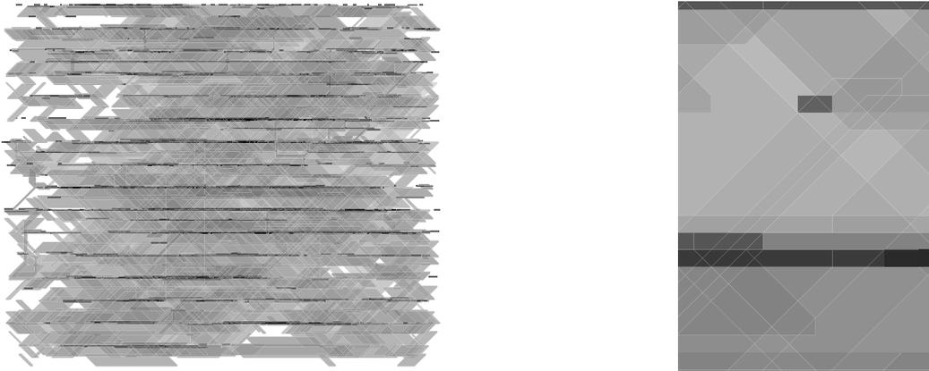
Figure 14: Overlay of flexibility polygons in VLSI routing. On the left is a full picture of a small chip, and on the right a zoom-in of a region of the picture of the left. Darker regions indicate more congested regions.
