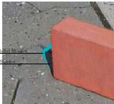
Figure 12: Real scene showing both, the real shadow casted by the brick and a virtual shadow casted by the brick. The virtual shadow is rendered using the estimated sun position.
