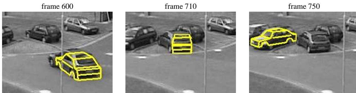
Figure 8: Tracking failures for the hatchback in the PETS 2001 test sequence: the wireframe turns clockwise at the level of the lamp-post (frame 600) and remains in that attitude (frame 710a); or else it “jumps out” of its correct pose (frame 730).
