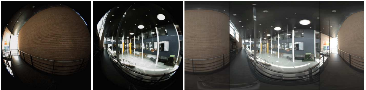
Figure 2: Left and center: two semi-spherical images acquired with a Sigma 180 degree field-of-view fish-eye lens in opposing directions. Right: the two semi-spherical images merged and mapped as a longitude-latitude light probe using HDRShop 2.09, [7].
