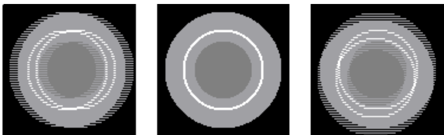
Figure 6.1: Interlacing artifacts: Serration, none (progressive) and line crawl
