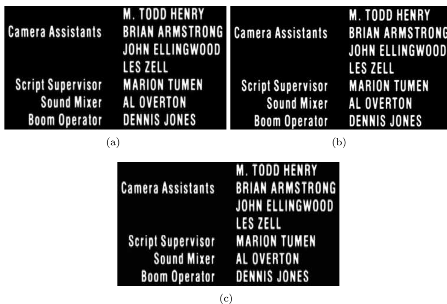
Figure 3.5: The sequence Credits has rolling end titles and the output of our variational MC deinterlacer in (a) is practically indistinguishable from the progressive original in (b) when viewed as video but appears a bit smoother as still (due to de-noising). The result of variational MA deinterlacing shown in (c) is also the second best performing deinterlacer on Credits and it does look quite good as still but has severe flickering when played.
