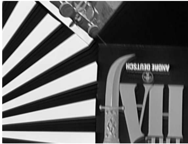
Figure 3.8: Variational motion compensated deinterlacing of the sequence BBC3 (cutout shown). A few artifacts are seen in the still, but they are not observed during playback. The motion in BBC3 is rotation around an axis in the lower left corner of the frame.
