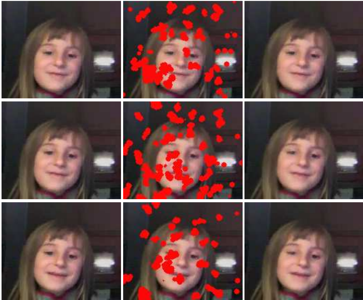
Figure 7: On the first column, frames 7,8 and 9 of the original Manon sequence. The second column shows the corresponding degraded frames and the last column the results of the color inpainting using Energy (E_2, E_3, E_4) .
